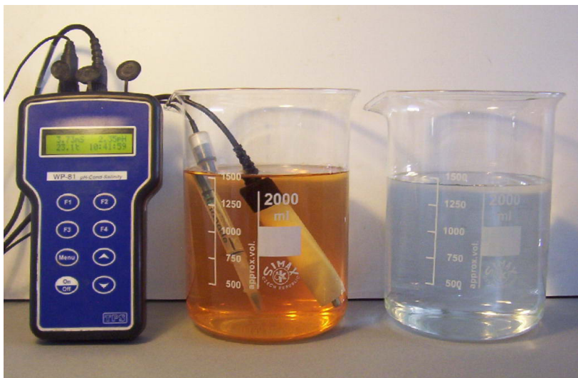
The difference between the raw pit water containing a high metal load and the pit water after treatment.
